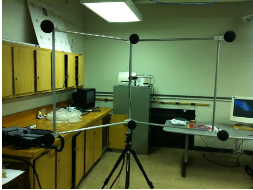
(a) The array of six microphones used to locate sound sources emitting arbitrarily time-dependent acoustic signals.
