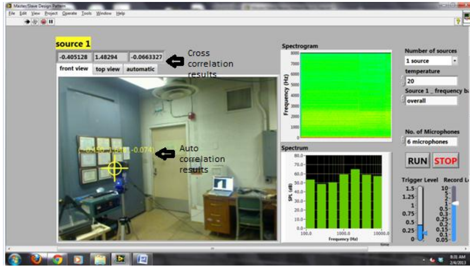
Figure 5.3 (b): Speaker kept at a left to the Microphones with cross-correlation and Auto-correlation results.
